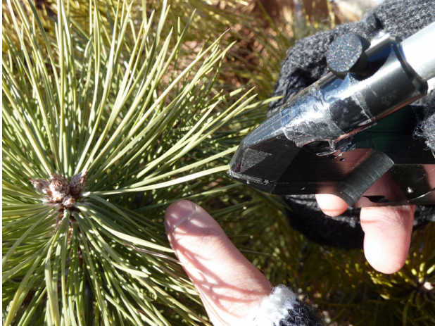
Figure 8 – leaf clip used for sampling pine needle reflectance (see Figure 7 ). The clip contains a bifurcated optical fiber that can measure reflected radiation on samples less than 1mm diameter within five seconds and is an example of specialized spectrometer foreoptics developed for capturing dynamic regulatory processes even in narrow plant leaves.
