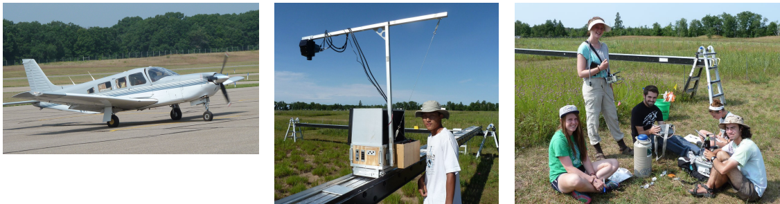
Figure 13. Field measurements of spectral diversity and biodiversity by airborne (a) and field (b) spectrometry, along with leaf-level measurements of reflectance and plant traits (c) at Cedar Creek, Minnesota. Figures: J. Gamon
