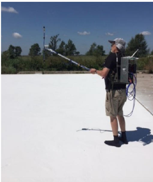
Figure 1. A field spectrometer being used to sample a uniform painted target during and aircraft overflight. In this case, proximal remote sensing is being used to obtain surface reflectance and correct for atmospheric effects using the Empirical Line Correction (ELC) method, as described in Wang et al. 2021. Note how the foreoptic (fiber optic mounted on a pole) is held at a distance (to avoid confounding effects of shadows). Dark clothing avoids casting reflected radiation on the calibration target. From Wang et al. 2021
