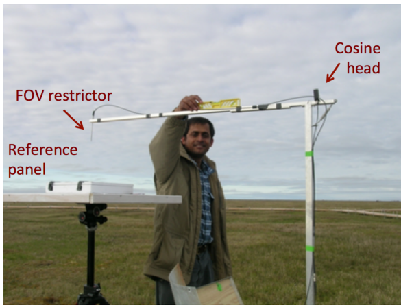
Figure 12 - Conducting a cross-calibration of a dual-detector spectrometer (UniSpec DC, PP Systems, Amesbury MA, USA) with an upward-looking fore-optic (fiber optic with cosine head, right arrow) and a downward looking fore-optic (fiber optic with FOV restrictor, left arrow) pointed at a reference panel. Cross-calibration corrects for changing sky conditions and enables accurate reflectance calculation, even under clouds. With this setup, two reference panels (a primary and secondary standard) are being compared to obtain the second term in eq. 6. Leveling of the sensors and panel helps standardize sampling geometry.
