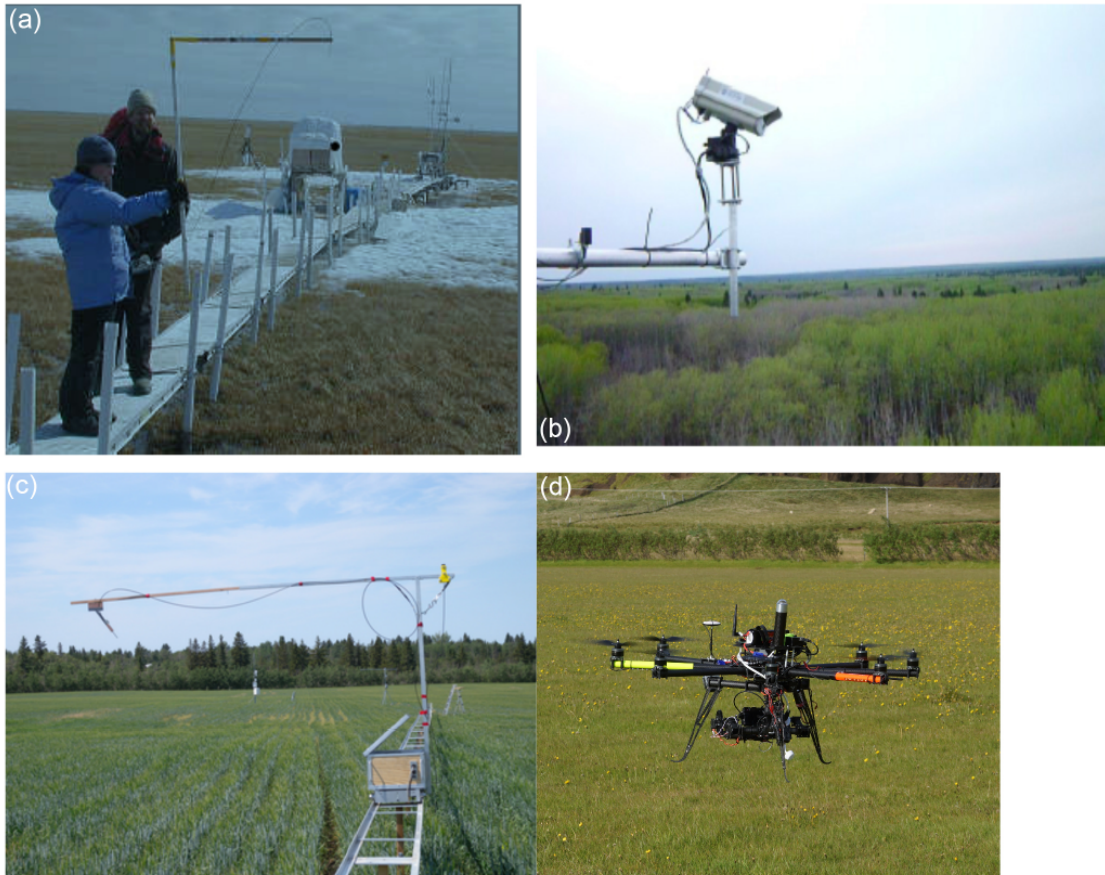
Figure 2. Examples of proximal optical sensing using spectrometers on a variety of platforms, including a) hand sampling, b) tower-mounted, c) tram-mounted, and d) UAV-mounted instruments. From Gamon et al. 2015.
